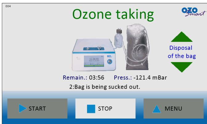
Bag is emptied with the pressure – 121.4 mBar (underpressure)
